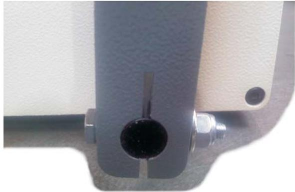
Tighten so that the two halves of the handle clamp down onto the shaft.
